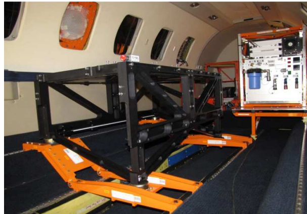
Figure 10: Empty LIDAR rack mounted upon seat rails
