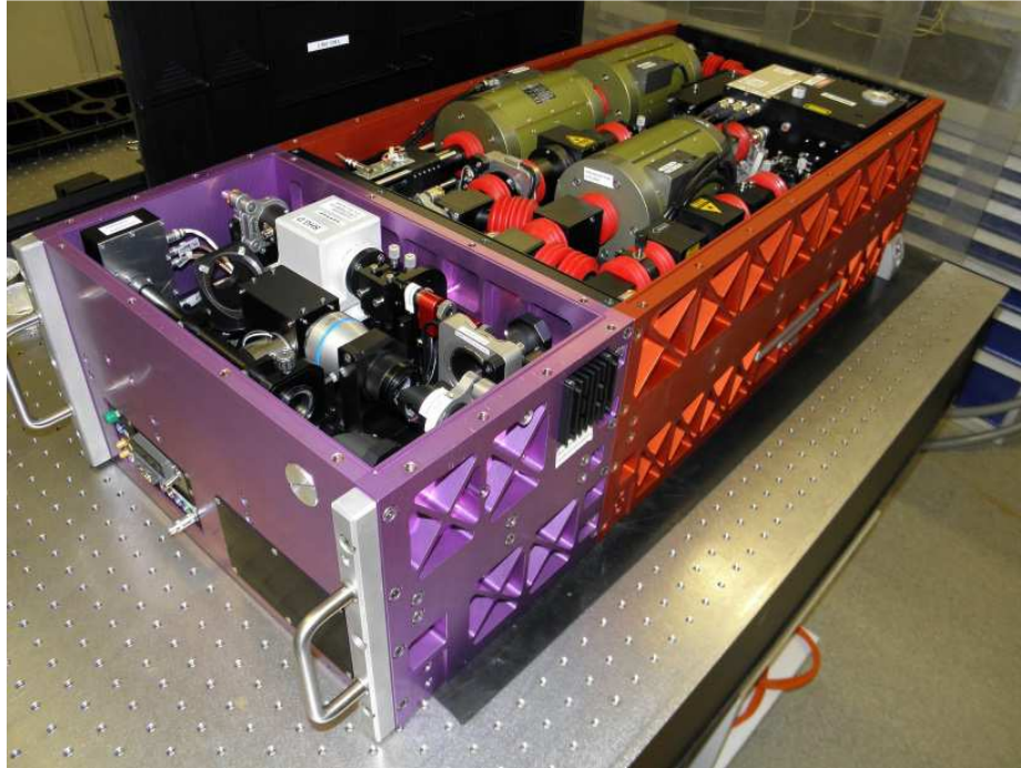
Figure 5: The DLR lidar transmitter with THG (front) and IR high power laser (rear)
