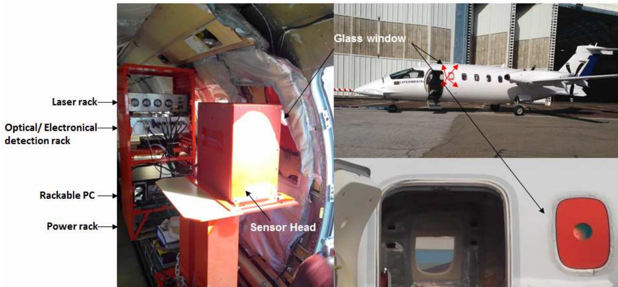
Figure 7 : Lidar anemometer installation on board P180.
