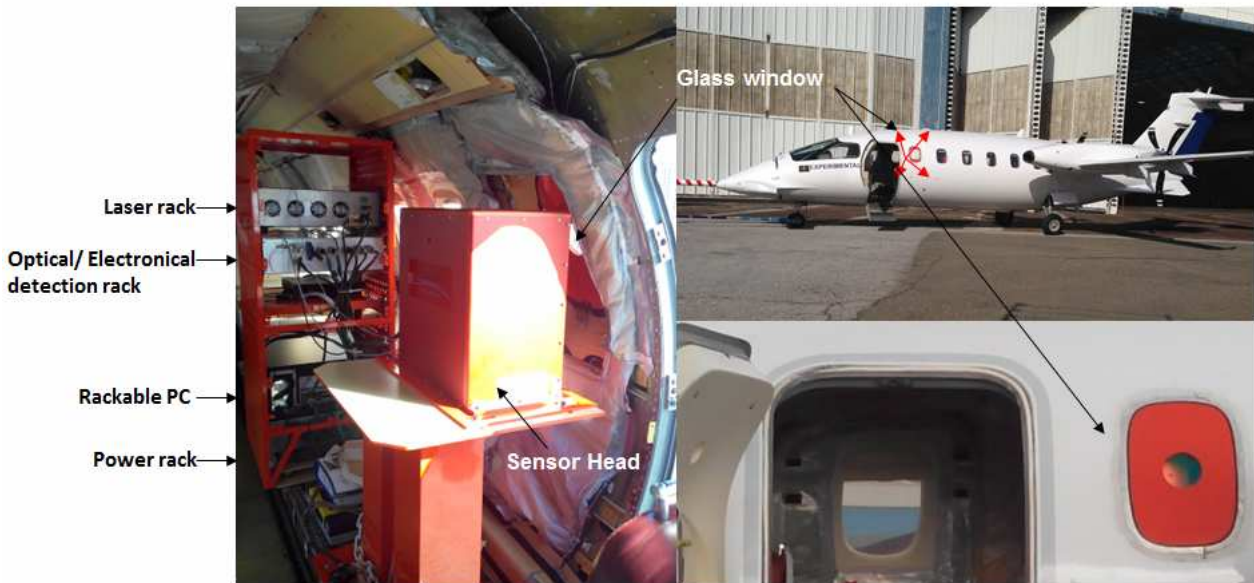
Figure 7 : Lidar anemometer installation on board P180.
