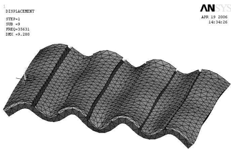
Fig. 13. Result of the modal analysis: deformed shape of the (8;0) mode at f=35.6\text{kHz} .
