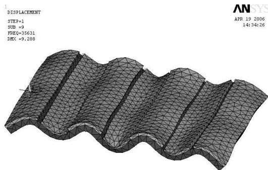
Fig. 11. Result of the modal analysis: deformed shape of the (8;0) mode at f=35.6kHz
