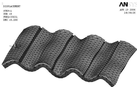
Fig. 11. Result of the modal analysis: deformed shape of the (8;0) mode at f=35.6\text{kHz}
