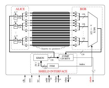
Fig. 5. Optimized cryptographically secure shield
