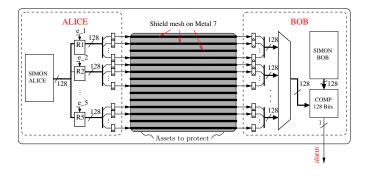
Fig. 3. Unoptimized cryptographically secure shield
