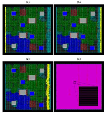
Fig. 8. Shield logic part (detail of Fig. 7(b)) in yellow. (a) ALICE, (b) BOB, (c) SHIELD INTERFACE, (d) shield mesh lines in M7 (with zoom)
