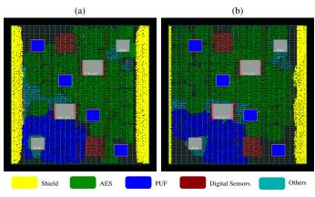
Fig. 7. Layout of the circuit (560  $\mu$ m  $\times$  560  $\mu$ m) with 30% core utilization rate. In yellow, the shield logic, for (a) non-optimized and (b) optimized logic
