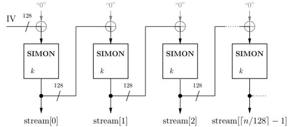
Fig. 6. Mode of operation of the SIMON block (keyed with  $k$ ), for the generation of the random data stream flowing through the mesh lines
