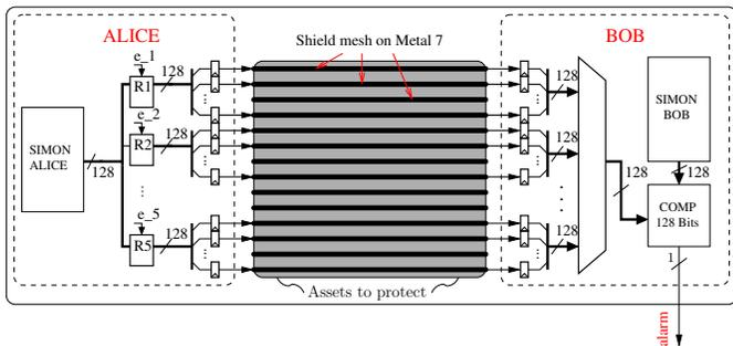
Fig. 3. Unoptimized cryptographically secure shield
