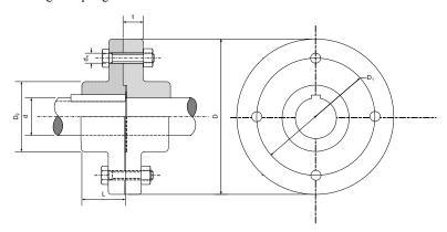
Table 1 shows the main design variables used in the example with their initial sets and types. Out of the 14 design parameters selected, seven are continuous variables whereas seven are discrete. The discrete variables may have additional defined attributes such as different material properties related to a specific bolt/flange material. Additional nomenclature related to the symbols used in the design model is presented in Appendix.
