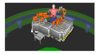
Fig. 5. Figure representing the same task as Figure 3 but planned with a simple RRT (Rapidly-exploring Random Tree [21]). The robot passes really close to the human.
