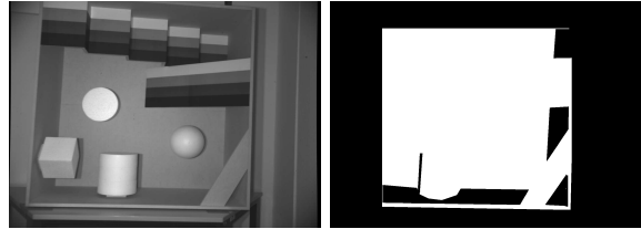
Fig. 12: The left image(left) and the mask that excludes inter-reflections (right) of the HCIBox dataset [17].
