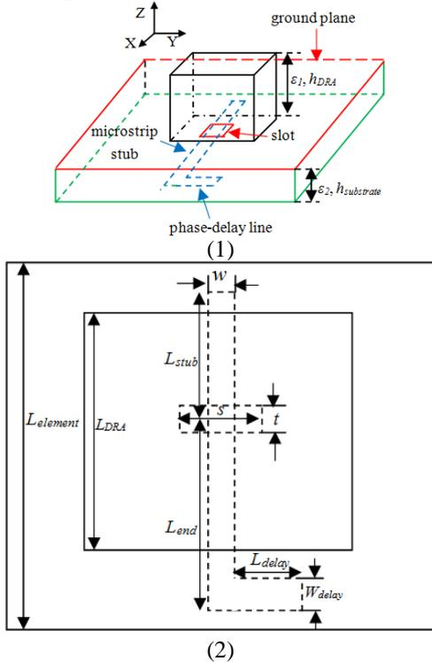
Fig. 3. DRA element design: (1) semi-sectional view, (2) top view;  $\epsilon_1=10$ ,  $\epsilon_2=4.4$ ,  $h_{DRA}=0.52\text{mm}$ ,  $h_{substrate}=0.15\text{mm}$ ,  $L_{element}=2.5\text{mm}$ ,  $L_{DRA}=1.2\text{mm}$ ,  $L_{end}=0.8\text{mm}$ ,  $L_{stub}=0.875\text{mm}$ ,  $s=0.79\text{mm}$ ,  $t=0.37\text{mm}$ ,  $w=0.28\text{mm}$ ,  $W_{delay}=0.2\text{mm}$ .
