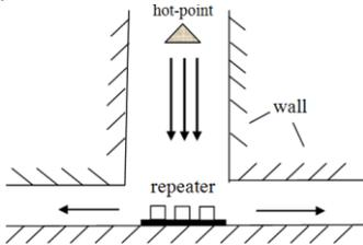
Fig. 1. Typical passive repeater relay in T-shape corridor.
