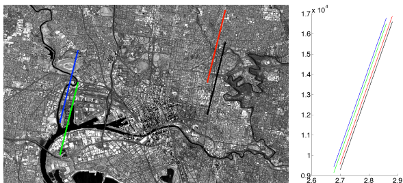
Figure 4: The RPC functions allow to draw the epipolar curves for a pair of images u and v (approx. 16000 \times 40000 pixels). The left image shows four epipolar curves plotted in the domain of image v , they correspond to four points located near the edges of the image u . The range of altitudes considered is h \in [-200, 3000] meters. The right image shows the same epipolar curves placed closer to facilitate the comparison.
