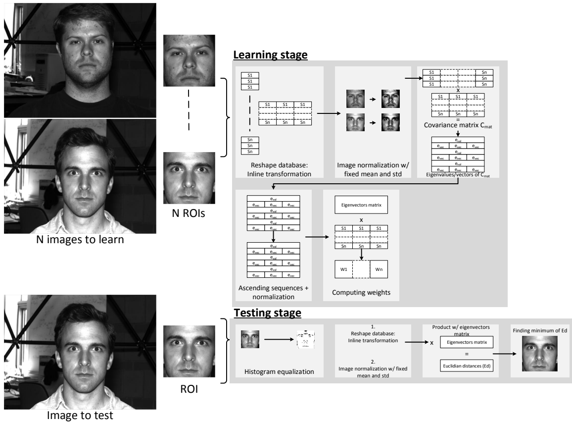
Figure 1: Basic face recognition flow based on eigenfaces
