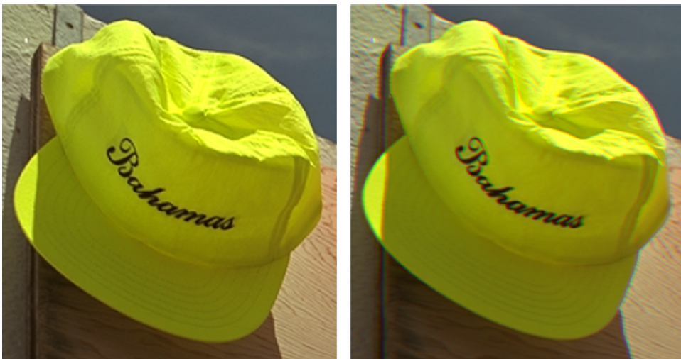
Fig. 13. Fragments of distortion-free (left) and distorted (right) image with chromatic aberrations.
