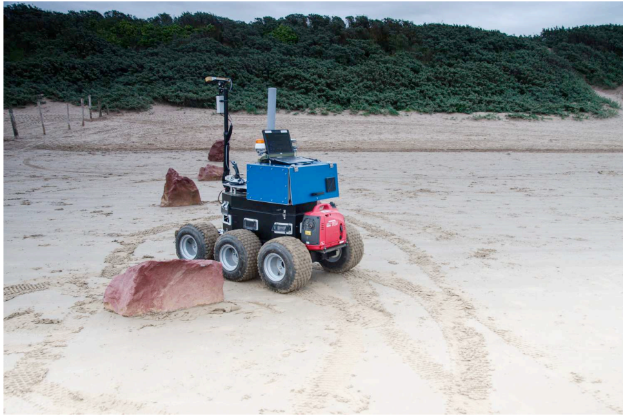
Figure 15: RoboVolc at Weston Beach performing obstacle avoidance manoeuvres
