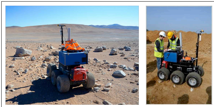
Figure 4: Seeker platform –Robovlc provided by BAE Systems. Bumblebee Stereo-pair mounted on the forward facing mast. Generator for extended operations mounted on the rear of the vehicle. D.P.G.S (ground truth testing) and Wi-Fi antenna in the centre.
