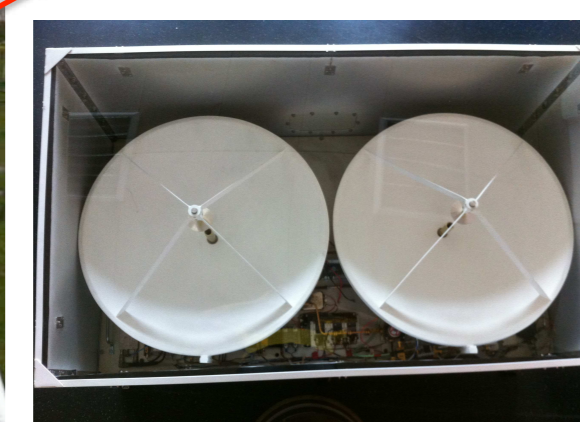
Blower: Remove water remaining on the radome
