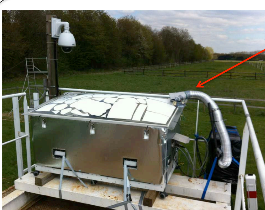
Blower: Remove water remaining on the radome
