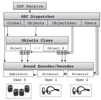
Figure 3: BlenderCAVE associated Sound Rendering Engine architecture implemented in Max/MSP. *objectUser* messages are used to allocate sound sources (Objects) to specific sets of Users. Sounds related to Object N for instance will here be rendered only in Users' headsets through the binaural engines embedded in the Sound Encoder/Decoder module. (See Figure 4 for associated messages)
