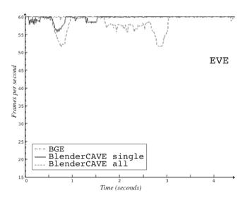
Figure 7: Enhanced frame-rates with respect to simulation time on the EVE system running the BGE, a single standalone Blender-CAVE Master (*BlenderCAVE single*), and a multi-screen Master/Slave Blender-CAVE instance (*BlenderCAVE all*) on 8 rendering nodes.
