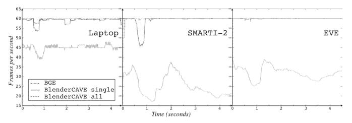
Figure 6: Frame-rates with respect to simulation time on three different architectures running the BGE, a single standalone BlenderCAVE Master (*BlenderCAVE single*), and a multi-screen Master/Slave BlenderCAVE instance (*BlenderCAVE all*). Laptop multi-screen run involves 2 BlenderCAVE windows (Master and Slave) on a single screen. SMART-I2 multi-screen run involves 4 instances on a single computer. EVE multi-screen run involves a BlenderCAVE instance on each of the 8 rendering nodes.
