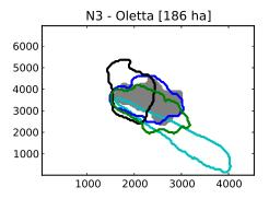
**Figure 4.** Case of the Oletta fire (21 August 2004; N3 in the Appendix) as observed (burned area in grey) and simulated by the non-stationary Balbi model (blue), the stationary Balbi model (green), the Rothermel model (black) and the 3 % model (cyan).
