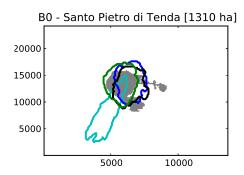
**Figure 5.** Case of the Santo Pietro di Tenda fire (1 July 2003; B0 in the Appendix) as observed (burned area in grey) and simulated by the non-stationary Balbi model (blue), the stationary Balbi model (green), the Rothermel model (black) and the 3 % model (cyan).
