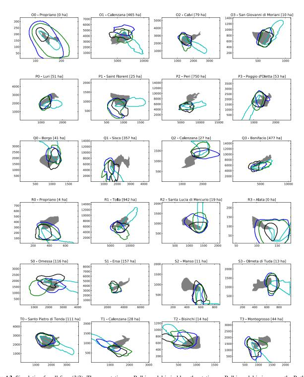
**Figure A3.** Simulation for all fires (3/3). The non-stationary Balbi model is in blue; the stationary Balbi model is in green; the Rothermel model is in black; the 3 % model is in cyan. The grey area is the observed final burned area. The coordinates are in metres.
