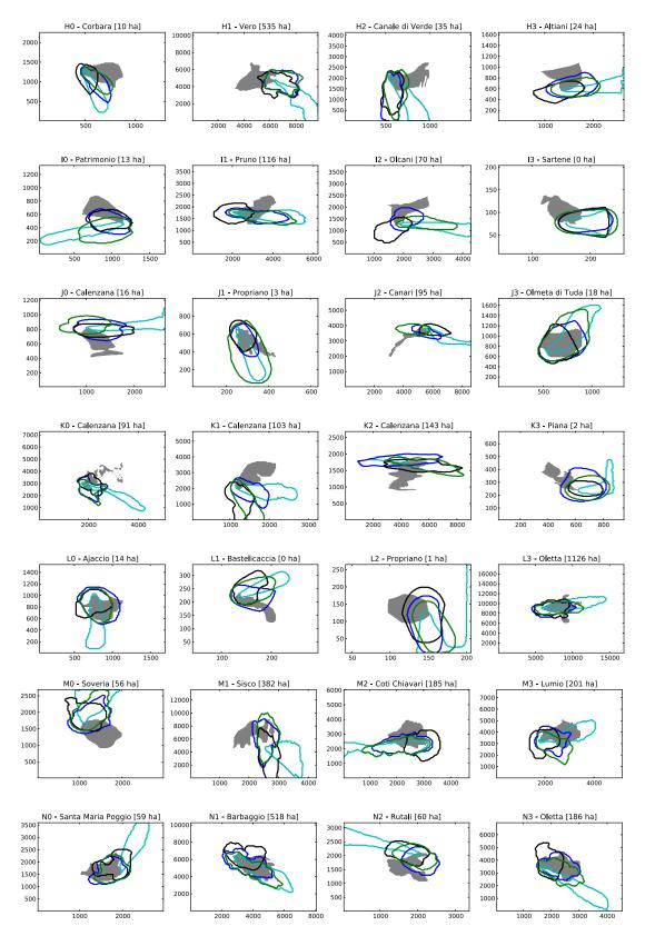
**Figure A2.** Simulation for all fires (2/3). The non-stationary Balbi model is in blue; the stationary Balbi model is in green; the Rothermel model is in black; the 3 % model is in cyan. The grey area is the observed final burned area. The coordinates are in metres.
