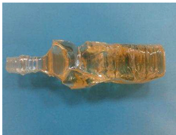
Fig. 1 Boule of Zn 100 MoO 4 single crystal with mass of 170.7 g and length of 95 mm grown by the low-thermal-gradient Czochralski process
