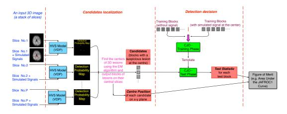
Fig. 2. Structure diagram of the multi-slice PCJO (msPCJO): the outputs of each step are highlighted in red.
