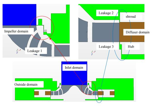
Figure 6. Regions modelled. Details of fluid leakages.
