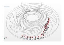
Figure 5. Diffuser measurement locations for probe traverse and unsteady calculations.
