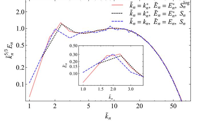
FIG. 4. (Color online) Compensated spectral density  $\tilde{k}_n^{5/3} \tilde{E}_n$  versus  $\tilde{k}_n$  from hydrodynamic turbulent DNS data. Two curves correspond to  $\tilde{k}_n = k_n$  and  $\tilde{E}_n = E_n$  or  $E_n^*$  and linearly spaced shells and the third curve corresponds to  $\tilde{k}_n = k_n^*$  and  $\tilde{E}_n = E_n^*$  and logarithmically spaced shells. The inset shows the spectral density at low wave numbers in the range of forcing scales.
