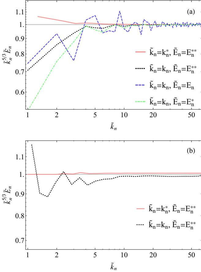
FIG. 3. (Color online) Compensated spectral density  $\tilde{k}_n^{5/3} \tilde{E}_n$  versus  $\tilde{k}_n$  for (a) linearly spaced shells  $S_n$  and (b) logarithmically spaced shells  $S_n^{\text{log}}$ . (a) The four curves correspond to  $\tilde{k}_n = k_n$  or  $k_n^*$  and  $\tilde{E}_n = E_n$  or  $E_n^*$ . (b) The curves corresponds to  $\tilde{E}_n = E_n^*$  and  $\tilde{k}_n = k_n$  or  $k_n^*$ .
