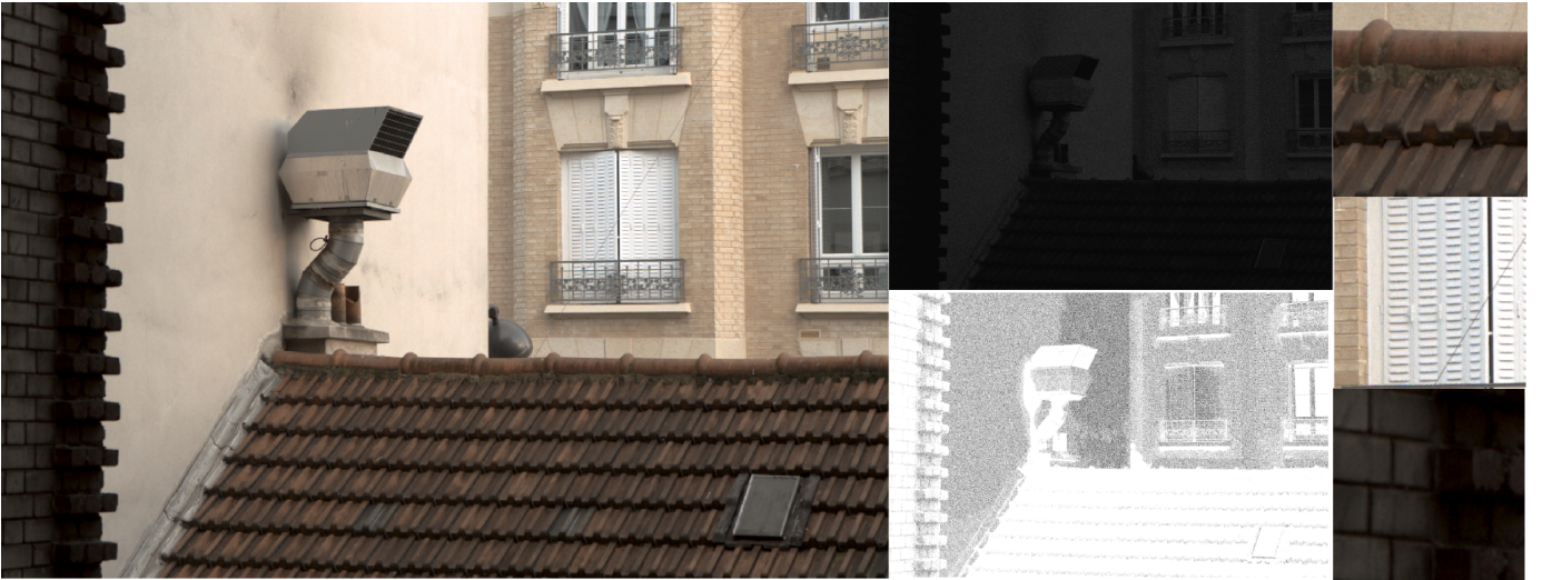
Fig. 10. Real data. Left: Tone mapped HDR image obtained by the proposed approach (11.4 stops). Middle top: Raw image with spatially varying exposure levels. Middle bottom: Mask of unknown (black) and known (white) pixels. In the regions with unknown pixels, the percentage of missing pixels varies between 25% to 40%. Right: Extracts of the scene.
