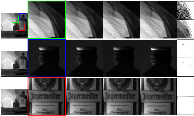
Fig. 9. Synthetic data. First column (top to bottom): Ground-truth with indicated extracts, result obtained by the proposed approach, result by Schöberl et al. [29] Second to fifth column (left to right): Ground-truth, result by the proposed approach, Schöberl et al. [29], Nayar and Mitsunaga [24]. Sixth column: Random (top) and regular (bottom) mask for each extract. Black represents unknown and white known pixels. The percentage of unknown pixels for the first extract is 65% (it is nearly the same for both the regular and non-regular pattern). For the other two extracts, most pixels are known (99%) so that the proposed method mostly performs denoising in these extracts.
