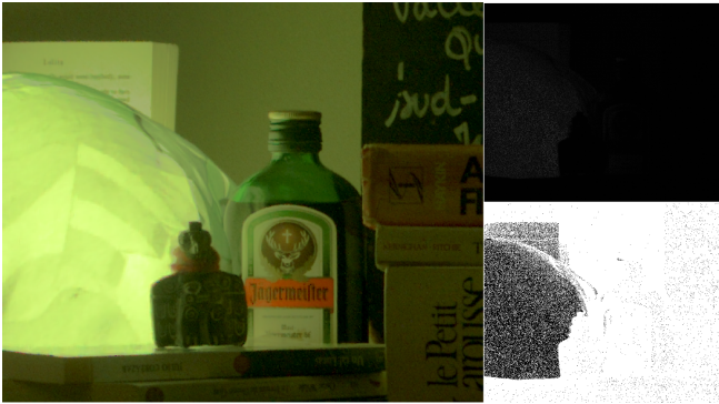
Fig. 7. Example of the acquisition of an HDR scene using spatially varying pixel exposures. Left: Tone mapped HDR scene restored from the raw image. Right top: Raw image with spatially varying exposure levels. Right bottom: Mask of correctly exposed pixels (white) and under or over exposed pixels (black).
