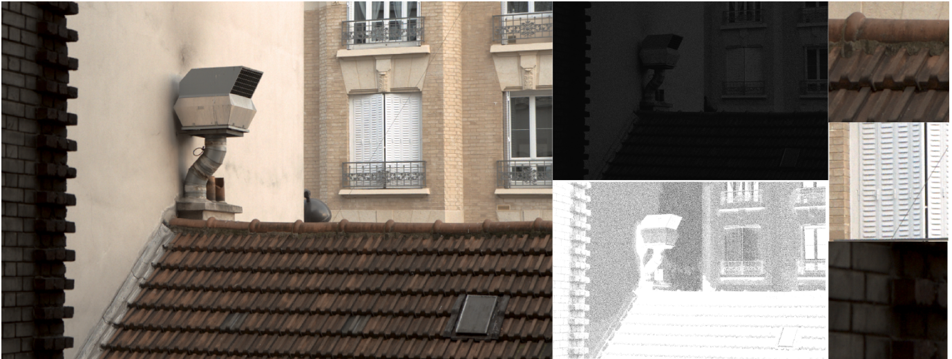
Fig. 10. Real data. Left: Tone mapped HDR image obtained by the proposed approach (11.4 stops). Middle top: Raw image with spatially varying exposure levels. Middle bottom: Mask of unknown (black) and known (white) pixels. In the regions with unknown pixels, the percentage of missing pixels varies between 25% to 40%. Right: Extracts of the scene.
