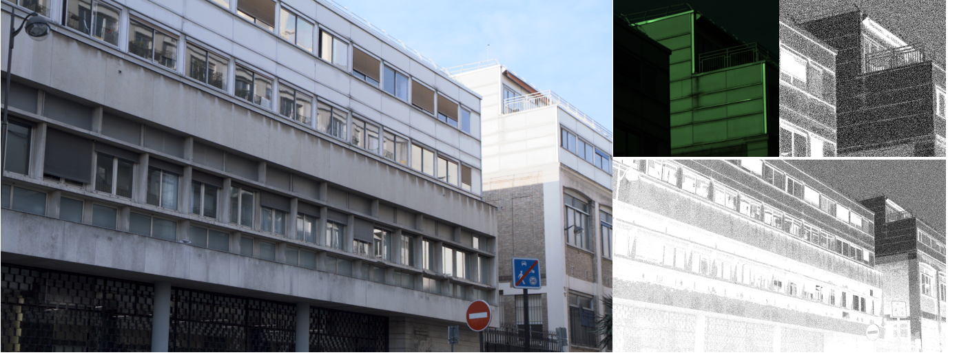
Fig. 11. Real data. Left: Tone mapped HDR image obtained by the proposed approach (15.6 steps). Right top: Extract of the building which is almost saturated by the tone mapping algorithm and mask of the corresponding extract. Right bottom: Mask of unknown (black) and known (white) pixels. In the brightest part of the building 73% of the pixels are unknown. Despite this fact, the reconstructed HDR image exhibits no visible artifacts.
