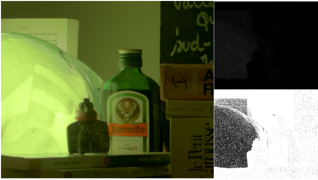
Fig. 7. Example of the acquisition of an HDR scene using spatially varying pixel exposures. Left: Tone mapped HDR scene restored from the raw image. Right top: Raw image with spatially varying exposure levels. Right bottom: Mask of correctly exposed pixels (white) and under or over exposed pixels (black).
