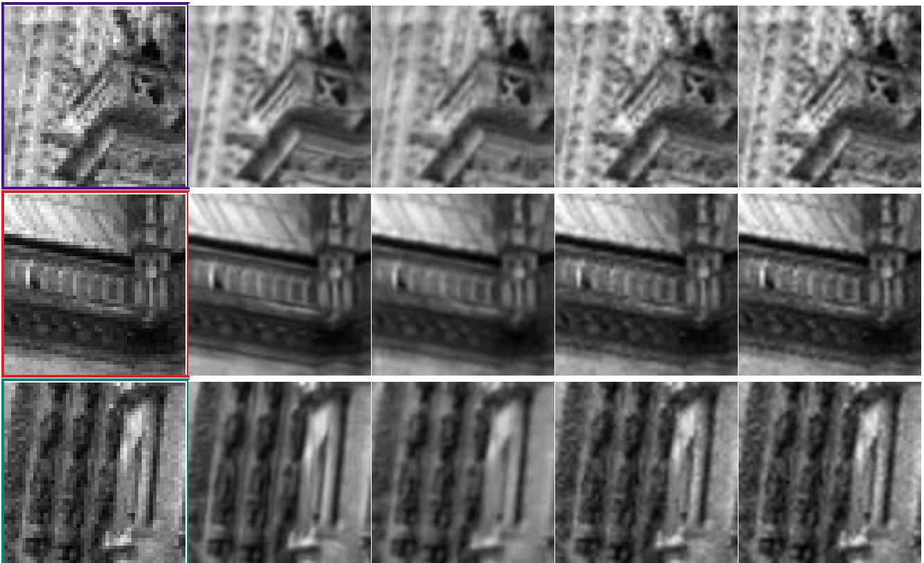
Figure 4. Real data. Zooming \times 2 . Interpolation of the green channel of a raw image (RGGB). Left to right: Input low-resolution image, result by HBE, PLE adapted to noise with variable variance [1], bicubic and lanczos interpolation.
