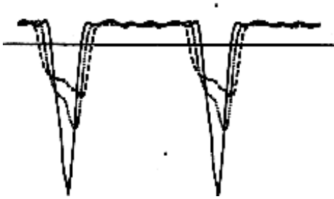
FIG. 2. Velocity of the bowing point as a function of time obtained on the digital bow under three conditions: \beta = 0.333 (dashed), \beta = 0.250 (dotted), and \beta = 0.293 (solid). The frequency is 70.16 Hz and two complete periods are shown. The absolute phase is arbitrarily chosen, to superpose the "slipping" pulse of the three curves.
