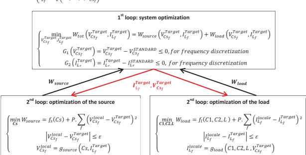
Figure 3. Architecture of the multilevel double loop optimization method
