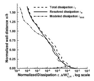
Figure 5: Comparaison of resolved, modelled and total dissipation  $\epsilon$ , suction side of the rotor at h/H = 50% and S/C = 80% (LES, grid M2).
