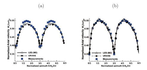
Figure 11: Time-averaged signals of axial velocity  $W_x/(\omega r)_{tip}$  at the rotor/stator interface at x=78 mm (nominal operating point): a) h/H=50% and b) h/H=80%. Experimental data are extracted from [14].
