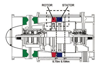
Figure 1: Axial view of the experimental compressor CME2. The plane at x=75 mm is located at 18% of the rotor chord downstream the rotor and the plane at x=194 mm is located at 50% of the stator chord downstream the stator.
