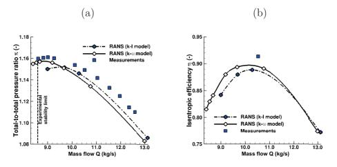
Figure 7: Unsteady RANS predictions of the compressor mean performance: a) total-total pressure ratio and b) isentropic efficiency. The experimental stability limit is found at  $Q = 8.57 \text{ kg.s}^{-1}$ .
