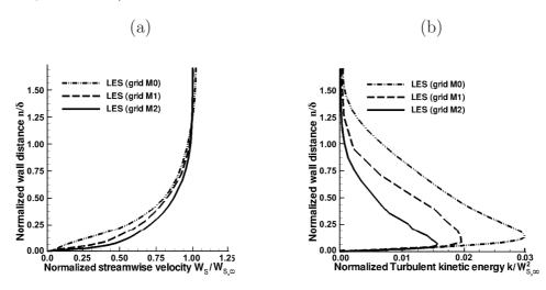
Figure 4: Influence of the mesh density on the time-averaged boundary layer profiles, rotor suction side at h/H = 50% and S/C = 80%: a) mean relative streamwise velocity  $\overline{W}_S$  and b) mean resolved turbulent kinetic energy  $\overline{k}$ .
