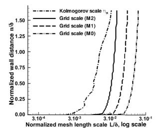
Figure 6: Comparaison of the Kolmogorov length scale  $\eta_k$  with the mesh length scale normalized with the boundary layer thickness  $\delta$ , on the rotor suction side, at h/H = 50% and S/C = 80% (LES, grid M2).
