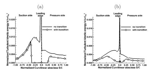
Figure 8: URANS predictions of the turbulent kinetic energy k in the boundary layer, at a wall distance of  $100\mu m$   $(n/\bar{\delta} \approx 0.03)$ , at h/H = 50%: a) rotor blade and b) stator vane.
