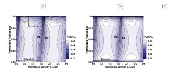
Figure 10: Time-averaged 2D flow fields of axial velocity  $W_x/(\omega R)_{tip}$  at the rotor/stator interface, at x=78 mm (nominal operating point): a) LES (grid M2), b) URANS with transition modelling. The dashed box points out the region where the tip leakage flow modifies the main flow.
