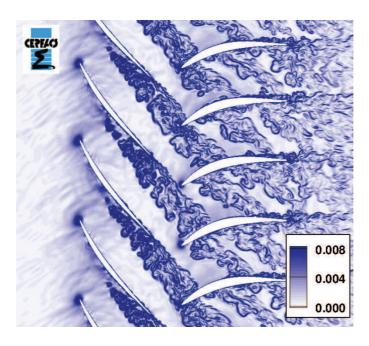
Figure 3: Instantaneous flow field shaded with density gradient  $grad\rho/\rho$  at h/H=90% (LES, grid M2). Flow comes from left to right and rotor rotates from bottom to up.
