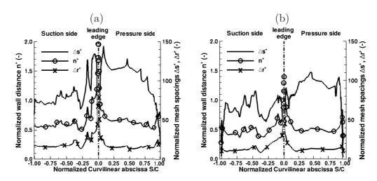
Figure 2: Averaged grid dimensions at wall (LES on mesh M2) around (a) rotor blade and (b) stator vane.
