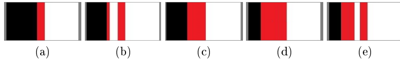
Fig. 5. Comparison of erosions of black color: (a) original image I , (b) erosion \varepsilon_{black}(I; B) using majority-based formulation (10), (c) erosion \varepsilon_{black}(I; B) using distance-based formulation (11). Let l be the width of the red line, the structuring element B is a square whose size is now between l and 2l . (d) iterated black erosion \varepsilon_{black}^2(I; B) using majority-based formulation, (e) erosion \varepsilon_{black}(I; 2B) using majority-based formulation.
