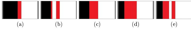
Fig. 5. Comparison of erosions of black color: (a) original image I , (b) erosion \varepsilon_{black}(I; B) using majority-based formulation (10), (c) erosion \varepsilon_{black}(I; B) using distance-based formulation (11). Let l be the width of the red line, the structuring element B is a square whose size is now between l and 2l . (d) iterated black erosion \varepsilon_{black}^2(I; B) using majority-based formulation, (e) erosion \varepsilon_{black}(I; 2B) using majority-based formulation.
