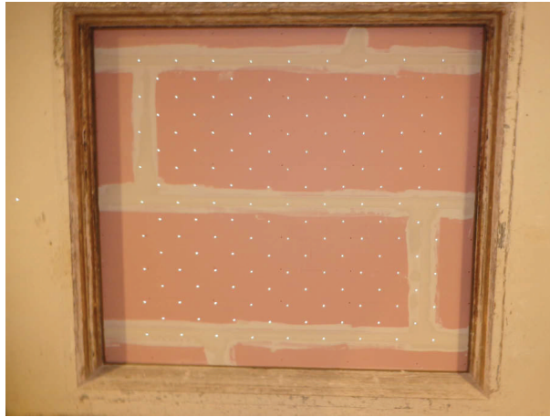
Figure 2: Double wall mounted in transmission test facility (as illustrated in Figure 1). Strips of retro-reflecting material (145 in total) are visible to enhance the optical reflection on a grid of locations on the wall, as required for the scanning laser vibrometry measurements.
