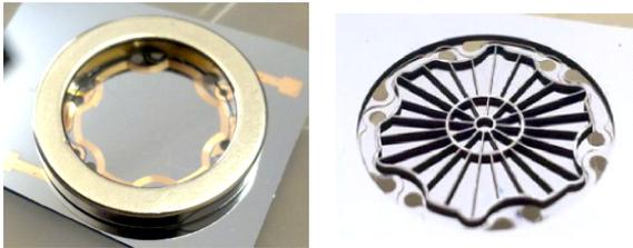
FIG. 8. Photos of the MEMS micro-speaker.
