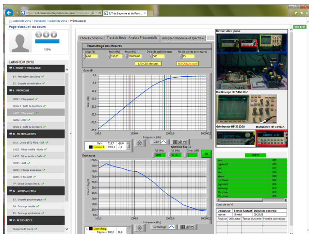
Fig. 2. Client rich interface showing a remote front panel: left) learning steps of the pedagogical scenario; center) results of experiment running (here Bode plots of a high-pass filter); right) video feedback of instruments, Top 10 list and queuing list of users.
