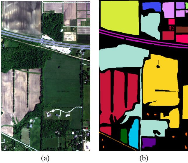
Figure 4: Indian Pines 2010 SpecTIR data.(a) RGB composition and (b) ground truth (for color legend, see Tab. 2). Unlabeled samples are in black.
