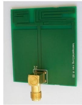
Fig. 1. First antenna topology, inspired by the World GSM Antenna.
