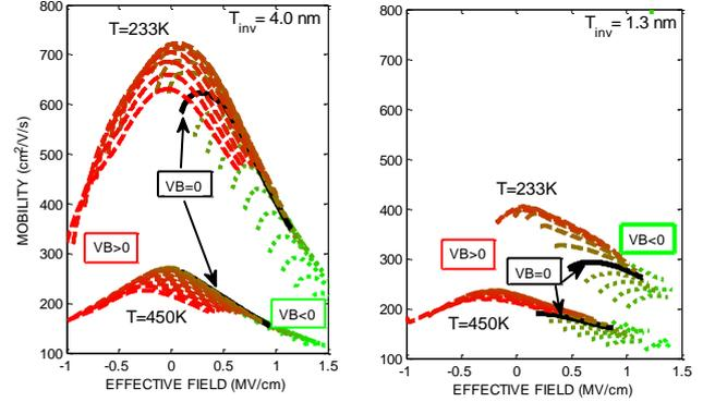
Figure 21: *n*FDSOI experimental effective mobility as a function of the effective field for VB in devices with  $T_{inv}=4.0$  nm (left) and  $T_{inv}=1.3$  nm (right). Effective field calculated using Eq.2 ( $\eta=0.62$ ).  $T=233$  K and 450 K. Measurements have been performed at zero VB (line), but also for  $V_B > 0$  (dashed lines) and  $V_B < 0$  (dotted lines).
