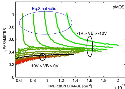
Figure 14: Extracted value of parameter  $\eta$  using Eq.3 in a pFDSOI device for various  $V_B$  ranging from -10 V to 10 V.  $T_{inv}=2.65$  nm.  $T=300$  K. In the front inversion regime ( $V_B > 0$ ),  $\eta \approx 0.36$  while in the forward regime ( $V_B < 0$ ),  $\eta$  varies significantly with  $V_B$ .
