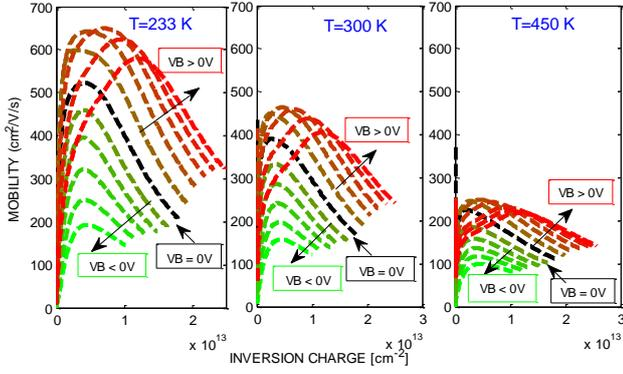
Figure 3: Effective experimental mobility as a function of the inversion charge for various VB ranging from -10 V to 10 V in steps of 2 V. nFDSOI device :  $T_{inv} = 2.65$  nm.  $T = 233, 300$  and  $450$  K.
