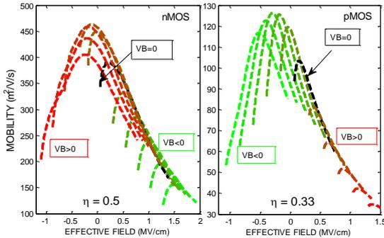
Figure 9: n- (left) and p- (right) FDSOI experimental effective mobility as a function of the effective field. VB ranging from -10 V to 10 V in steps of 2 V. Effective field calculated using Eq.2 ( $\eta=0.5$  for nFDSOI and  $\eta=0.33$  for pFDSOI).  $T_{inv}=2.65$  nm.  $T=300$  K.
