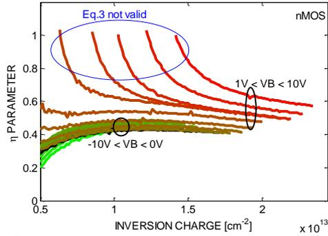
Figure 13: Extracted value of parameter  $\eta$  using Eq. 3 in a nFDSOI device for various  $V_B$  ranging from -10 V to 10 V.  $T_{inv}=2.65$  nm.  $T=300$  K. In the front inversion regime ( $V_B < 0$ ),  $\eta \approx 0.42$  while in the forward regime ( $V_B > 0$ ),  $\eta$  varies significantly with  $V_B$ .
