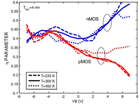
Figure 16: Extracted value of parameter  $\eta$  as a function of  $V_B$  in n- and pFDSOI devices for three different temperatures ( $T=233, 300$  and  $450$  K).  $\eta$  extracted using Eq.3.  $T_{inv}=4.0$  nm. Extractions have been done at  $V_G=2.5$  V.
