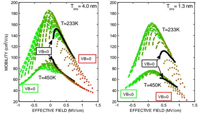
Figure 22: *p*FDSOI experimental effective mobility as a function of the effective field in devices with  $T_{inv}=4.0$  nm (left) and  $T_{inv}=1.3$  nm (right). Effective field calculated using Eq.2 ( $\eta=0.62$ ).  $T=233$  K and 450 K. Measurements have been performed at zero VB (line), but also for  $V_B < 0$  (dashed lines) and  $V_B > 0$  (dotted lines).
