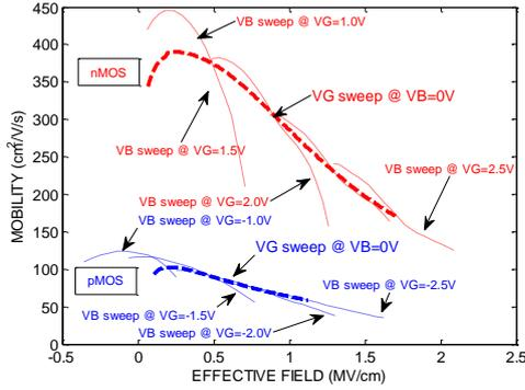
Figure 19: *n*- and *p*- FDSOI experimental effective mobility as a function of the effective field sweeping the back terminal or the gate terminal. Eq.2 have been used for the evaluation of the effective field with  $\eta=0.62$  for nFDSOI and  $\eta=0.5$  for pFDSOI devices.  $T_{inv}=2.65$  nm.  $T=300$  K.
