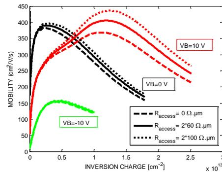
Figure 2: Effective experimental mobility as a function of the inversion charge for various  $\text{VB} (-10\text{V}, 0\text{V}, 10\text{V})$  corrected from access resistances (not corrected,  $2 \times 60 \Omega \cdot \mu\text{m}$  and  $2 \times 100 \Omega \cdot \mu\text{m}$ ). nFDSOI device :  $T_{\text{inv}}= 2.65 \text{ nm}$ .  $T=300 \text{ K}$ .
