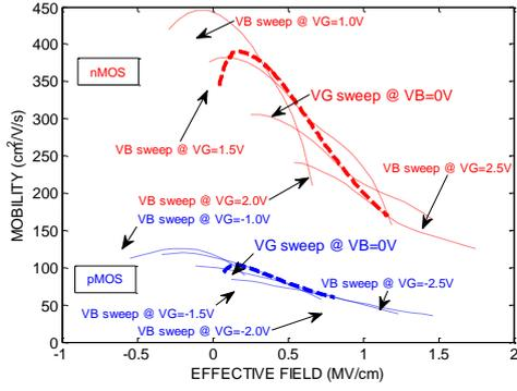
Figure 18: *n*- and *p*- FDSOI experimental effective mobility as a function of the effective field sweeping the back terminal or the gate terminal. Eq.2 have been used for the evaluation of the effective field with  $\eta=0.42$  for nFDSOI and  $\eta=0.36$  for pFDSOI devices.  $T_{inv}=2.65$  nm.  $T=300$  K.
