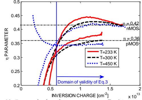
Figure 10: Extracted value of parameter  $\eta$  using Eq. 3 in n- and pFDSOI devices for various temperatures ( $T=233, 300$  and  $450$  K). nFDSOI device :  $T_{inv}=2.65$  nm. The domain of validity corresponds to the strong front inversion regime.
