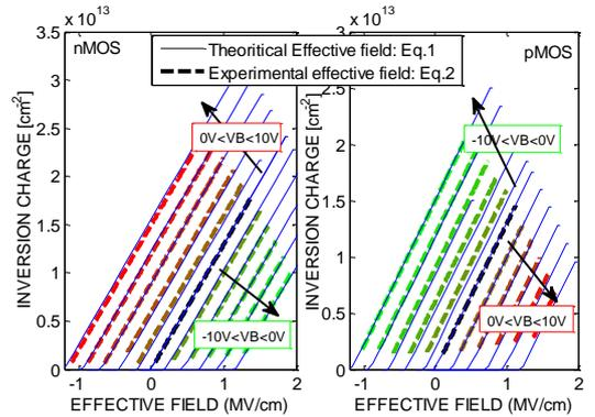
Figure 8: n- (left) and p- (right) FDSOI average electric field (Eq.2) assuming  $\eta = 0.5$  compared to the simulated theoretical average field (Eq.1).  $VB$  from  $-10$  V to  $10$  V in steps of  $2$  V.  $T_{inv} = 2.65$  nm;  $T = 300$  K.
