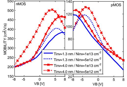
Figure 7: n- (left) and p- (right) FDSOI experimental effective mobility as a function of  $VB$  extracted for  $N_{inv} = 5e12$   $cm^{-2}$  and  $1e13$   $cm^{-2}$ . Two structures:  $T_{inv} = 1.3$  nm and  $4.0$  nm.  $T = 300$  K.
