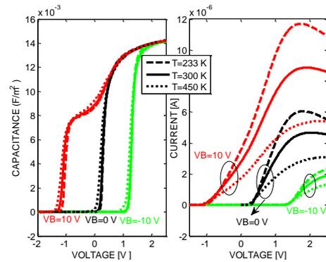
Figure 1: Gate capacitance (left) and drain current (right) as a function of the gate voltage for  $\text{VB}=-10, 0$  and  $10 \text{ V}$  and for various temperatures ( $T=233, 300$  and  $450 \text{ K}$ ) in a nFDSOI device:  $T_{\text{inv}}= 2.65 \text{ nm}$ .
