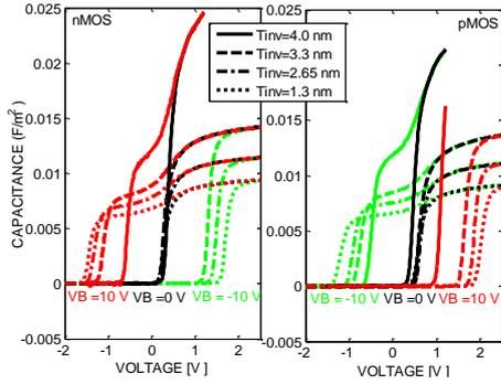
Figure 4: Gate capacitance as a function of the gate voltage for  $VB = -10, 0$  and  $10$  V in n- (left) and p- (right) FDSOI devices with  $T_{inv} = 1.3$  nm,  $2.65$  nm,  $3.3$  nm and  $4.0$  nm.  $T = 300$  K.
