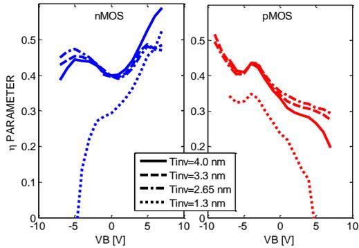
Figure 15: Extracted value of parameter  $\eta$  as a function of  $V_B$  in n- and p-FDSOI devices with various IL EOT (devices of figure 4).  $\eta$  extracted using Eq.3.  $T=300$  K. Extractions have been done at  $V_G=2.5$  V for devices with  $T_{inv}=2.65, 3.3$  and  $4.0$  nm and at  $V_G=1.2$  V for devices with  $T_{inv}=1.3$  nm.
