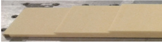
Fig. 1. Stepped sample before the pressing process (5, 10, 15mm thick)
