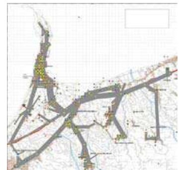
(b) Total traffic assigned to the road network during the day (line width proportional to traffic)
