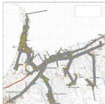
(b) Total traffic assigned to the road network during the day (line width proportional to traffic)
