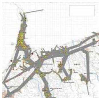
(b) Total traffic assigned to the road network during the day (line width proportional to traffic)
