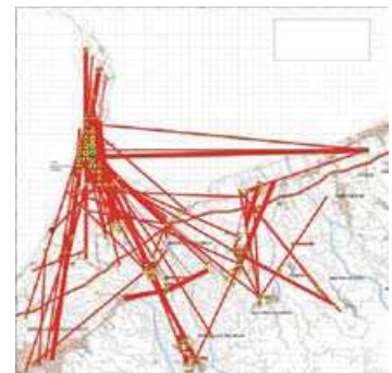
(c) Total origin/destination flows during the day (line width proportional to the number of movements)
