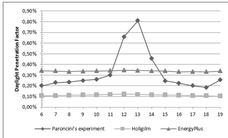
Fig. 11. Daylight Penetration Factor under the diffuser (June 27, 2006)
