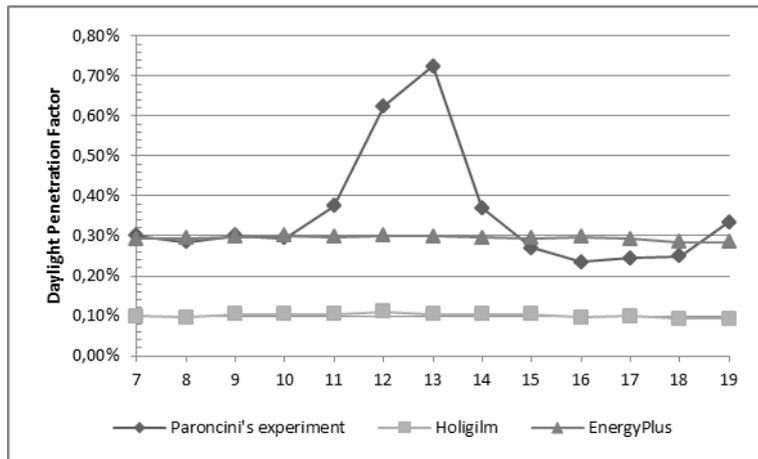
Fig. 10. Daylight Penetration Factor at sensor C (April 27, 2006)
