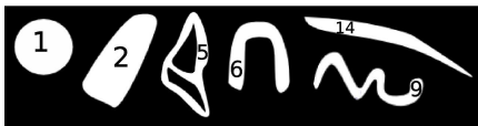
Figure 2: Geodesic elongation for different binary objects. The elongation values have been approximated to get integer values.
