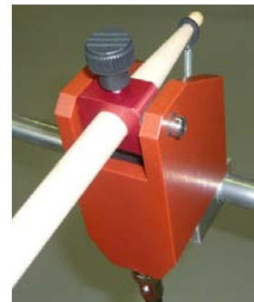
Fig. 4. Machined housing and "pin part"
