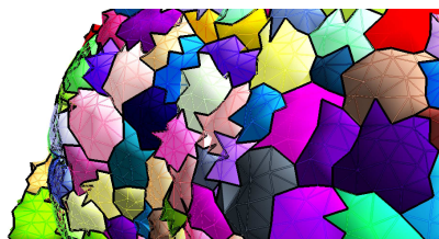
Figure 3: Surface triangles of the mesh of shoot apical meristem cells built from the tetrahedral mesh generated by Delaunay refinement.
