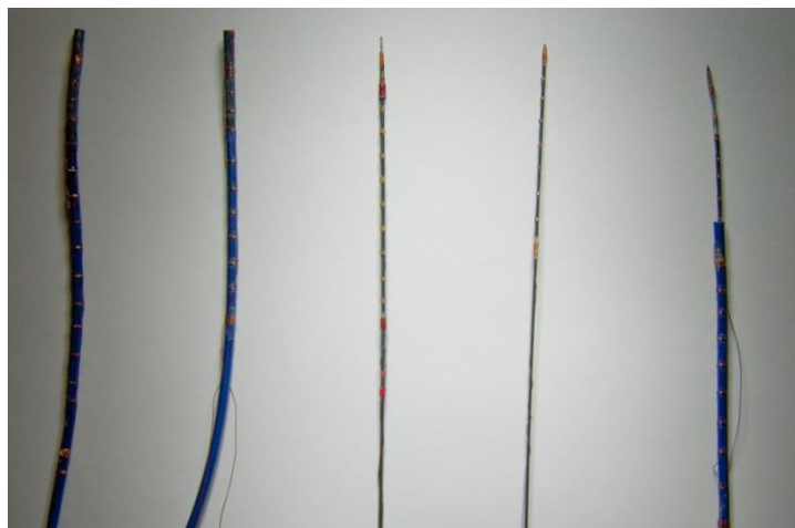
Fig 2 - Prototypes of different diameters and controllable shape. From left to right, (a) 6-Fr multi-stage active catheter, (b) single stage active catheter, (c) Multi directional active guidewire, (d) single stage active guidewire, (e) active guidewire combined with an active catheter.
