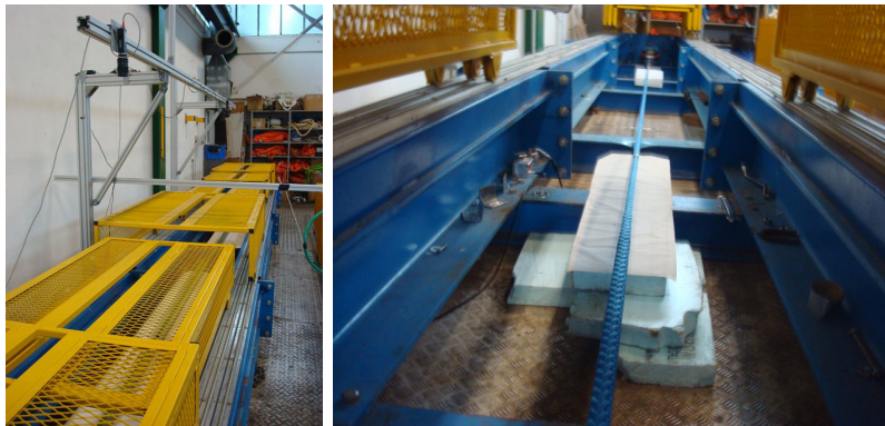
Figure 11: Test frame for rope tests. Left: Overview showing cameras above test frame. Right: Rope in place during test.
