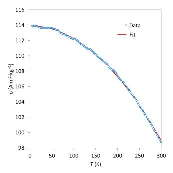
Fig. 2. Specific moment as a function of temperature for the  $Mn_{54}Al_{44}C_2$  alloy sintered at 923 K. The experimental data follow well a quadratic (without linear term) law.
