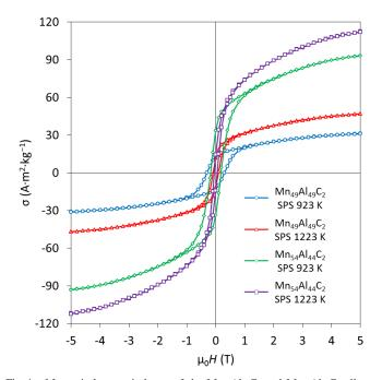
Fig. 1. Magnetic hysteresis loops of the  $Mn_{49}Al_{49}C_2$  and  $Mn_{54}Al_{44}C_2$  alloys sintered at different temperatures. The samples with higher coercivity have lower specific moment because of smaller content of the  $\tau$ -phase.
