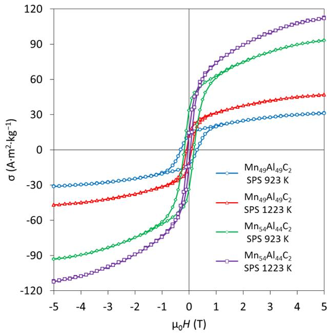
Fig. 1. Magnetic hysteresis loops of the  $\text{Mn}_{49}\text{Al}_{49}\text{C}_2$  and  $\text{Mn}_{54}\text{Al}_{44}\text{C}_2$  alloys sintered at different temperatures. The samples with higher coercivity have lower specific moment because of smaller content of the  $\tau$ -phase.
