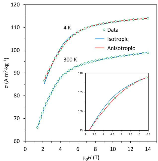
Fig. 4. Ahysteretic parts of magnetization curves for the  $\text{Mn}_{54}\text{Al}_{44}\text{C}_2$  alloy, sintered at 923 K, at different temperatures. Fitting to isotropic and anisotropic models for the approach to saturation. In the inset a magnified fragment of the 4 K curve illustrates the difference between the two approximations.
