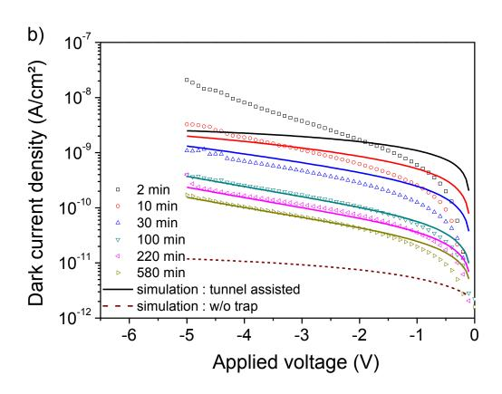
**Figure 10.** Dark current density versus applied voltage, for several annealing duration using simple trap assisted recombination model a) or using trap assisted recombination model accounting for tunneling b). Parameters are the same of figure 15.
