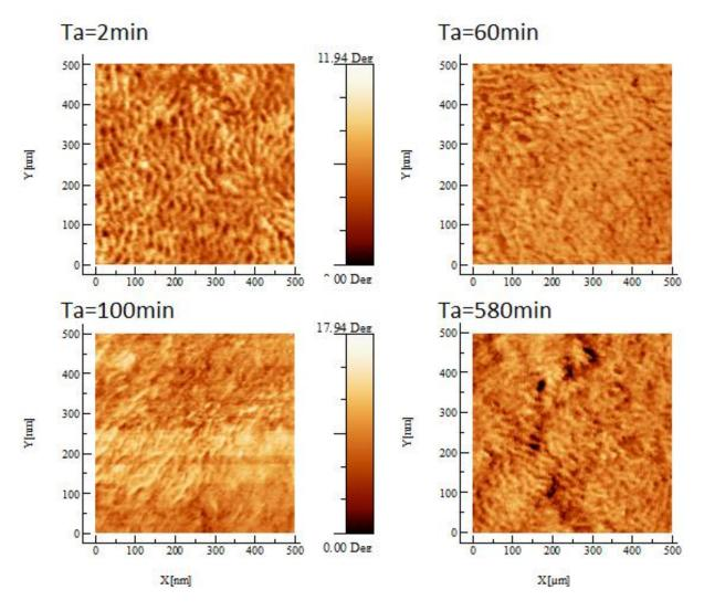
**Figure S1.** Atomic Force Microscope (AFM) phase measurement in tapping mode performed on the P3HT:PC<sub>60</sub>BM blend surface, obtained with different annealing duration (2min, 60min, 100min and 580min). The blend layer was spin coated on the ITO coated glass substrate.
