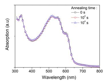
**Figure S3.** Absorption spectra of P3HT:PC<sub>60</sub>BM blend layer with 95% of CB and 5% of DIO. The crystallization order of the film is unchanged along with the annealing.
