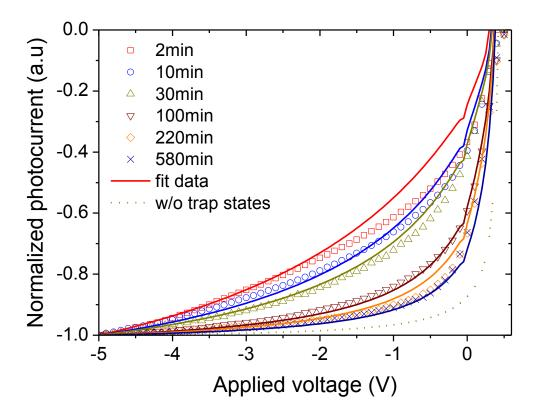
**Figure 8.** Comparison between experimental and simulated photocurrent I-V curves for the different annealing steps. The evolution of the interface volume fraction  $V_f$  (extracted from AFM images) is taken into account in the simulation, as well as the evolution of the band tail characteristic energy  $E_0$  (extracted from EQE experiments).
