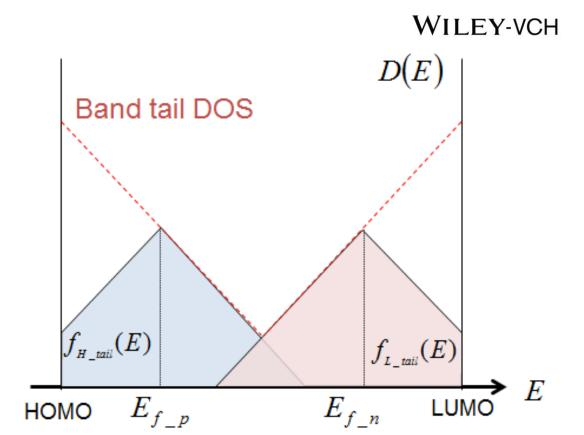
**Figure S5.** Band tail density of states in the blend band gap with the occupation probability of the energy state. The gap states are described by an exponential density.  $E_{f\_p,n}$  represents the quasi Fermi level energy.
