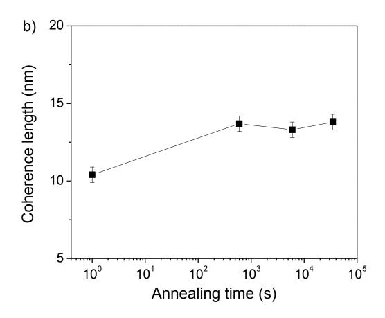
**Figure 2.** a). Schematic representation of the orientation of ordered P3HT domains with side chains perpendicular to the substrate; b). Coherence length extracted from X-rays diffraction spectra at the identified (001) peak using the Scherrer formula.
