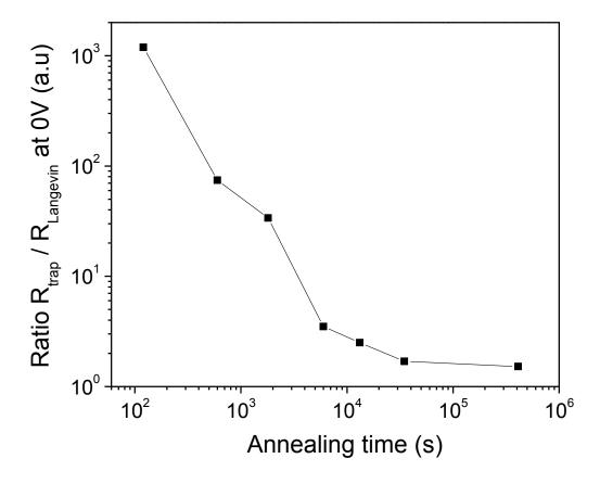
**Figure 9.** Calculation of the ratio between the SRH recombination and the Langevin recombination terms at short circuit condition as function of the annealing time. For high band tail states, Langevin recombination can be neglected whereas for optimized efficiency, the Langevin term is of the same order of magnitude than the SRH term.
