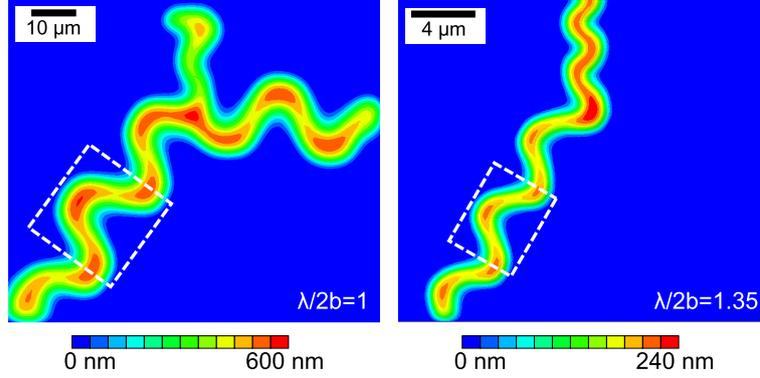
Figure 5: Out of plane displacement for two different TC morphologies obtained by numerical simulations, with  $E = 329$  GPa: (left)  $h = 100$  nm,  $\sigma_0 = 2.5$  GPa,  $G_{Ic} = 0.477$  J.m $^{-2}$  resulting in an aspect ratio of 1.0; (right)  $h = 40$  nm,  $\sigma_0 = 3.1$  GPa,  $G_{Ic} = 0.4$  J.m $^{-2}$  with an aspect ratio 1.35.
