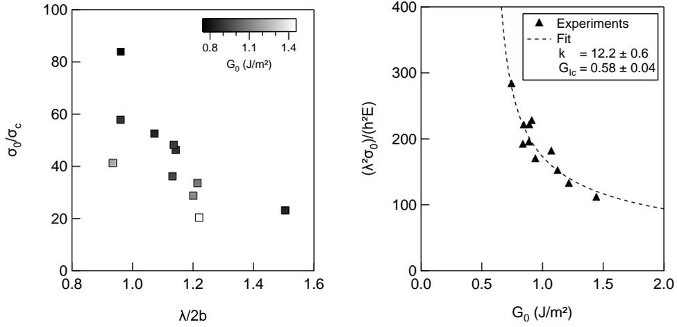
Figure 8: (left) measured loading ratio  $\sigma_0/\sigma_c$  as a function of aspect ratio  $\lambda/2b$  for a series of films with identical SiO<sub>2</sub>/Ag interface; (right) non-dimensional loading parameter for the experimental TC buckle as a function of total elastic energy prior rupture.
