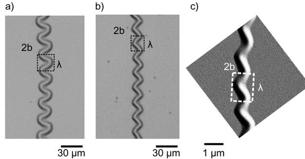
Figure 7: Microscopy photographs (a,b) and AFM phase image (c) for different values of  $G_0$  for the same interface, and hence same adhesion  $G_1^c$ . This series of images illustrate the variation of the aspect ratio  $\lambda/2b$  with  $G_0/G_1^c$ .
