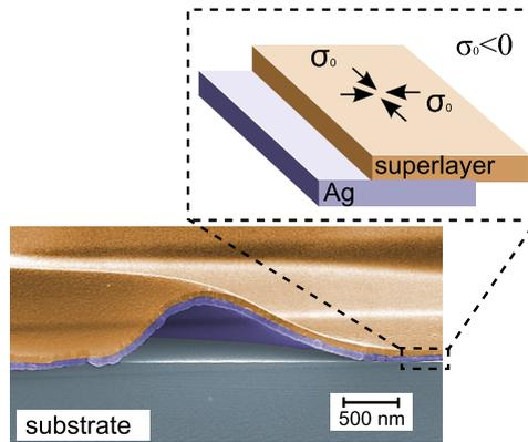
Figure 1: Scanning electron micrograph of a buckled thin film (cross-section). The stack consists of 80 nm of molybdenum and 80 nm of silver on a silicon wafer.
