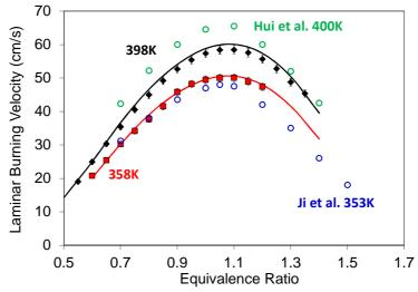
Figure 2: Laminar flame velocities as a function of equivalence ratio for *n*-propyl-benzene at two fresh gas temperatures (358 and 398 K). Symbols are experimental data and lines simulations performed using the LLNL model. Empty symbols refer to experimental data from Hui et al. [4] and Ji et al. [5].
