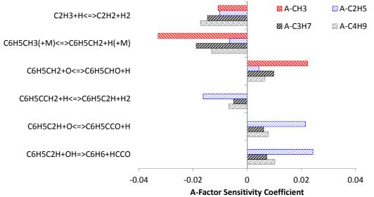
Figure 6: A-sensitivity factor analysis on the flame speed of four alkyl-benzenes: toluene, ethylbenzene, *n*-propyl-benzene, *n*-butyl-benzene using modified heat capacities for nitrogen.  $T_u = 358$ ,  $\Phi = 1$ , flame temperature is 2337 K ± 1 K for all the case. The symbol A-represents the phenyl group  $(C_6H_5-)$ .
