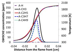
Figure 7: Concentration profiles of the  $C_6H_5CH_2$  radical in proximity of the flame front for the five fuels considered in our analysis. The symbol A-represents the phenyl group ( $C_6H_5$ –). (For the benzene flame, the concentration of benzyl radical is negligible).
