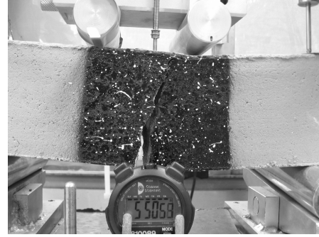
Figure 1: Beam test and cracking mode
